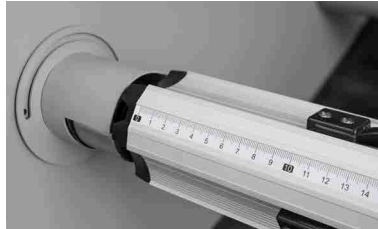
Millimeter scale on the shafts for the right positioning of the rolls
