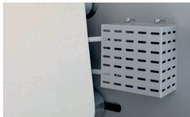
Felt belt automatic tracking system by PLC
