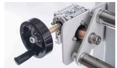
Fabric tensioning adjustment
