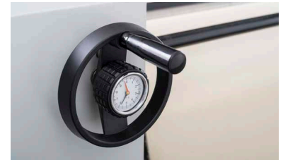
Felt tensioning adjustment with pressure gauge
