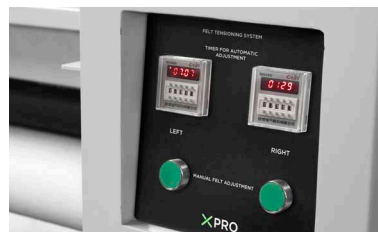
Felt belt automatic tracking system
