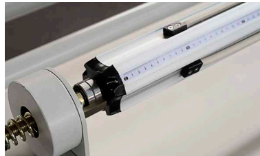
Millimeter scale on the shaft for the right positioning of the rolls
