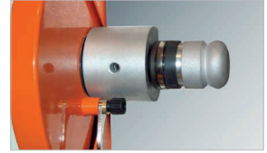
Braking assembly for the cutting blade suggested for cutting fabrics and other particular materials (optional)
