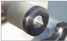
Pneumatic locking system of spindle
