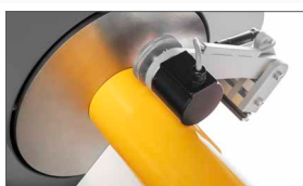
Encoder for measuring the rewind meters
