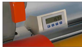
Digital display for cutting measurement (optional)
