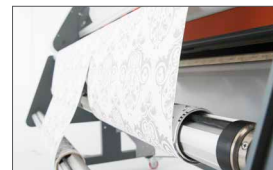
Front rewinding system: it rewinds the cut media up to three smaller rolls (optional for Miura Plus 160)
