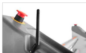
Wi-Fi antenna to communicate data with Flexa Cloud
