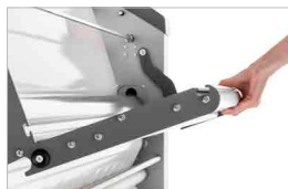
Swing-up feed table for quick set-up
