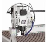
For cutting the CNC router is equiped with **professional spindle**. 2kW power is well balanced with machine design and power of vacuum. Maximum speed is 24000 RPM, thanks to double ceramic bearings, hardened shaft, balancing and forced cooling, the spindle can run in such speed for the full shift.
