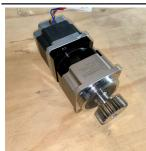
To ensure accuracy and smooth diagonal movement you will find **planetary gearboxes** in X and Y axis - which is not usual in this price range.
