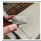
For measuring of tool length. The automatic Z sensor is standard for COMAGRAV ECO.
